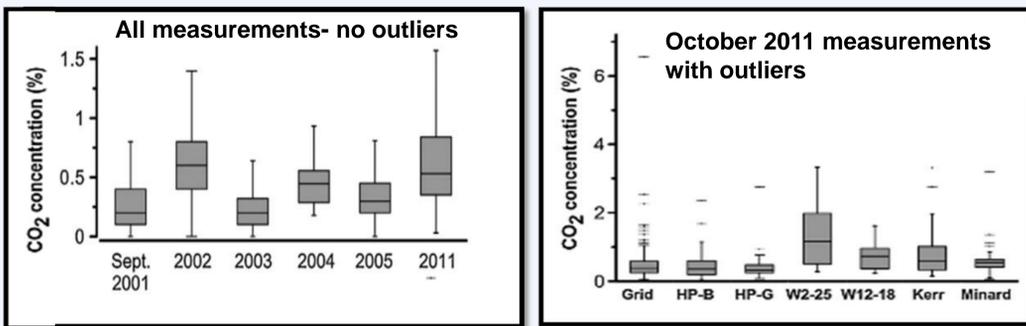
(Left) What would have happened at Weyburn in 2002, 2004, or 2011 if baseline was only measured in 2001, 2003 or 2005? (Right) If the boxes are used for assessment, the background site (Minard) has less CO<sub>2</sub> than the Kerr Farm, W12-18, and W2-25. If outliers are considered, the background site has less CO<sub>2</sub> than the grid. Such assessments would have led to false leakage claims at the Weyburn field using the current thinking on leakage attribution.
