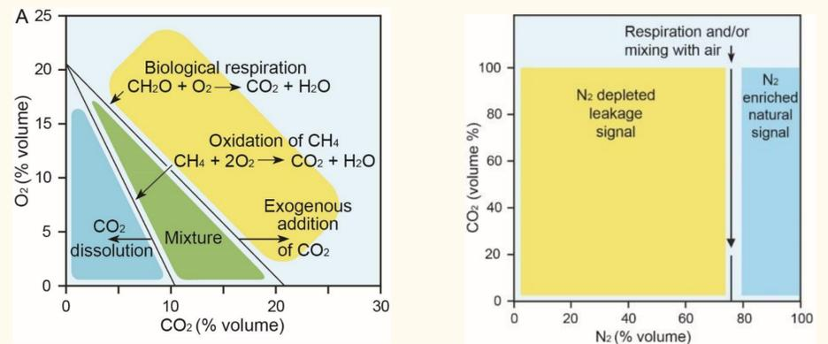
Respiration is the main cause of environmental variability. This process can be represented by one simple line on a graph using process-based (PB) ratios (Romanak et al., 2012). Leakage will simply fall to the right of the respiration trend.
