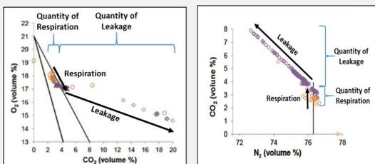
Monitoring of simulated leakage at the ZERT site (Romanak et al., 2014) shows that a PB method can separate natural from leaked CO<sub>2</sub>. Can this method increase the accuracy of emissions quantification and delineate areal extent of leakage?
