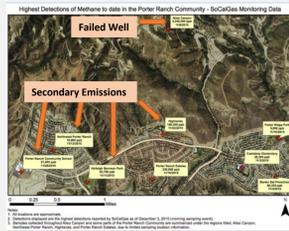
The well failure resulted in several areas of surface flux far from the well. How will these types of emissions be identified as leakage, quantified, and monitored for effective remediation at CO<sub>2</sub> storage sites?
