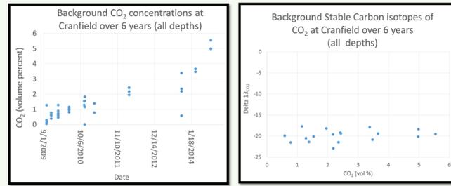
Six years of background monitoring at Cranfield shows increasing CO<sub>2</sub> concentrations yet no change in carbon isotopes (injectate = -5 per mil) suggesting that increased respiration is causing increased CO<sub>2</sub>.
