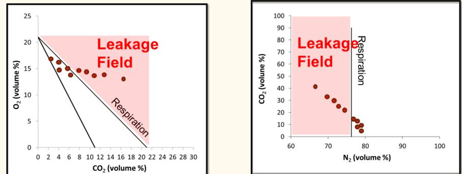
Because the method is simple and has a graphical interface, the public can understand and even implement it themselves in real-time. "Baseline" is now defined as the respiration line. Anything plotting to the right is potential leakage and can be further assessed. In this way, the threshold for action is clear, universal, and simply-defined with no ambiguity or complexity to confuse stakeholders.
